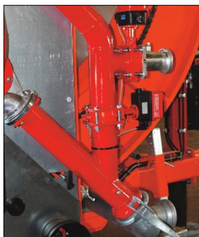
Electric valve motorisation
