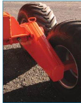
Articulated tandem axle (adjustable track)
