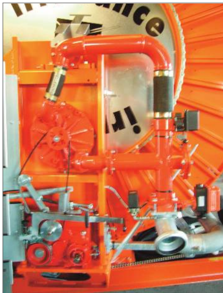
Turbine motorization VA
