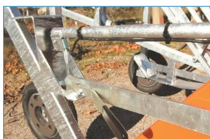
End-of-winding sensor and frame lock
