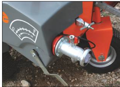
Speed regulation through by-pass
