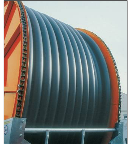
Twin drum drive chains
