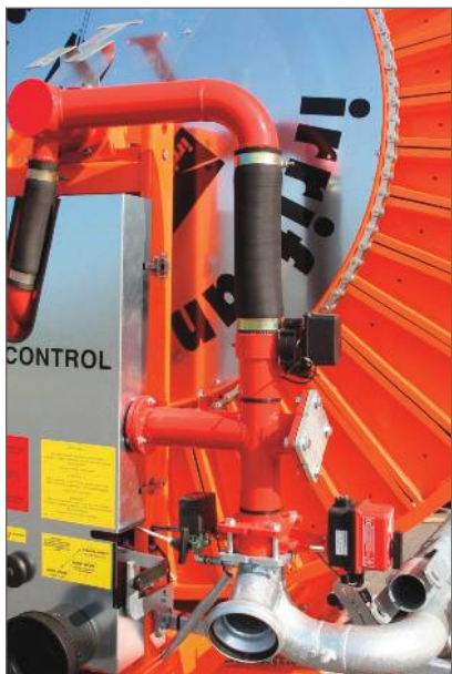
Supply tubing with integrated valve
