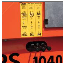
Side hydraulic distributor (stabilizer + frame + lifting frame and rotating frame control)
