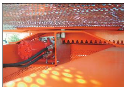
Hydraulic rotation of the turntable
