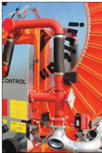
Automatic shut-off valve VA
