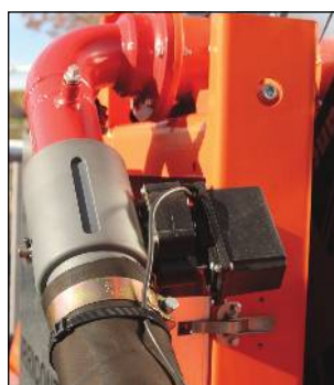
Butterfly valve controlled by electric motor
