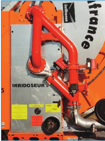
Motorization (cast aluminium turbine)
