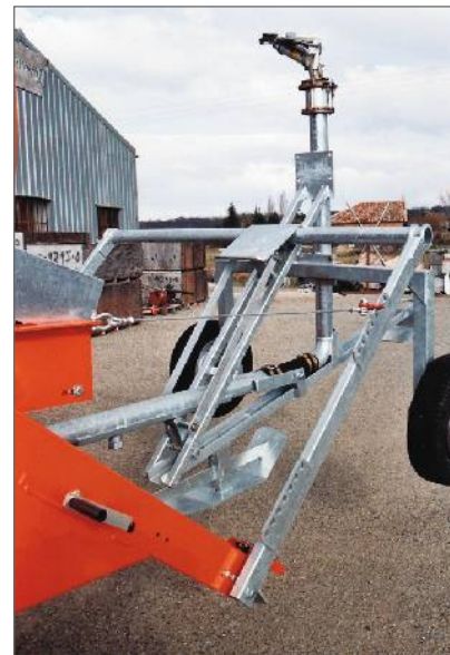
Automatic trolley lifting preventing crop-washing damages
