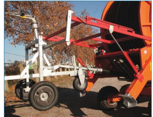
Articulated trolley series 2000 & hydraulic lifting frame
