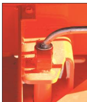
Mechanical rotation of the turntable with automatic locking
