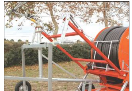
Automatic trolley hooking
